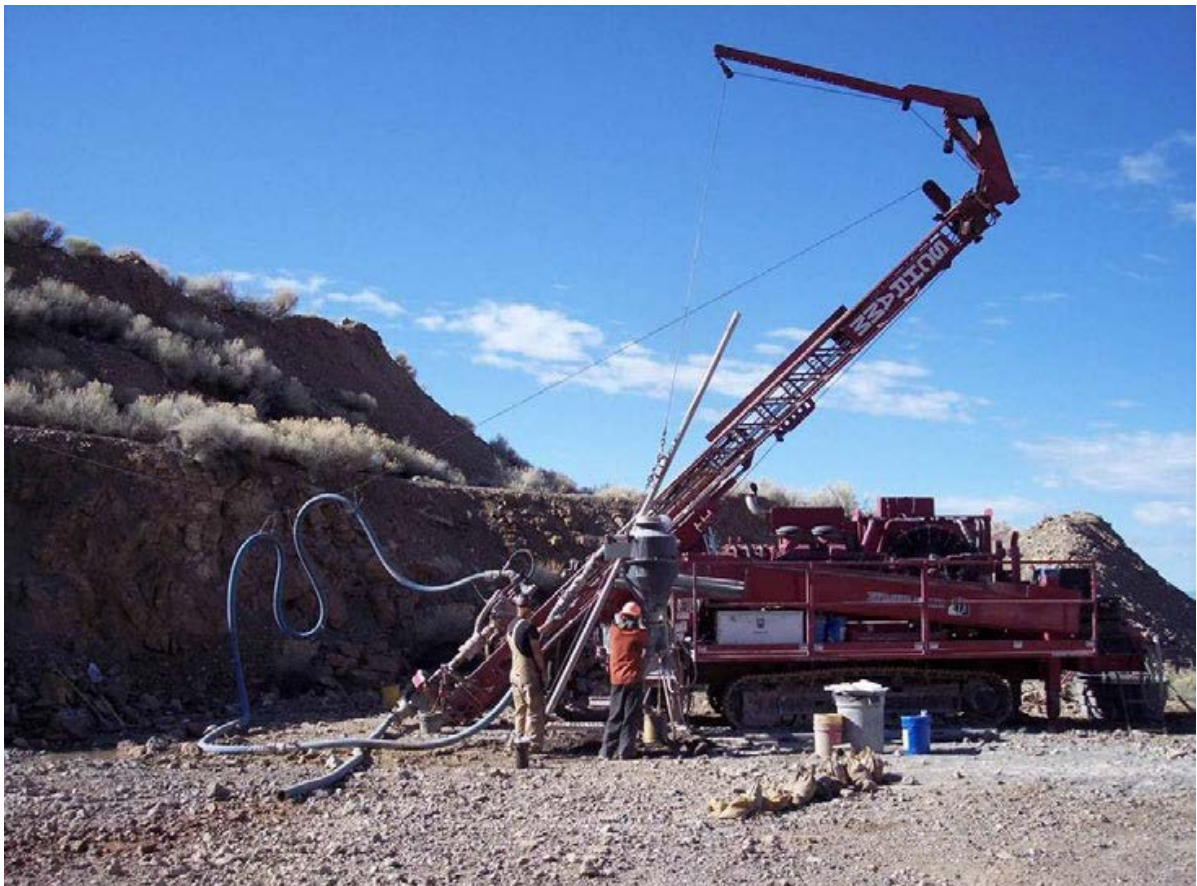
Figure 10-2: Reverse Circulation Track-Mounted Drill Rig at Taylor
