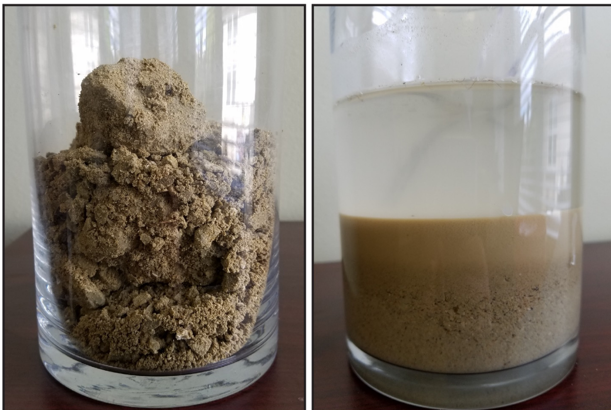
Figure 13-2 Images of Typical ROM Ore (Left) and After Soaking/Agitating in Water (Right)
