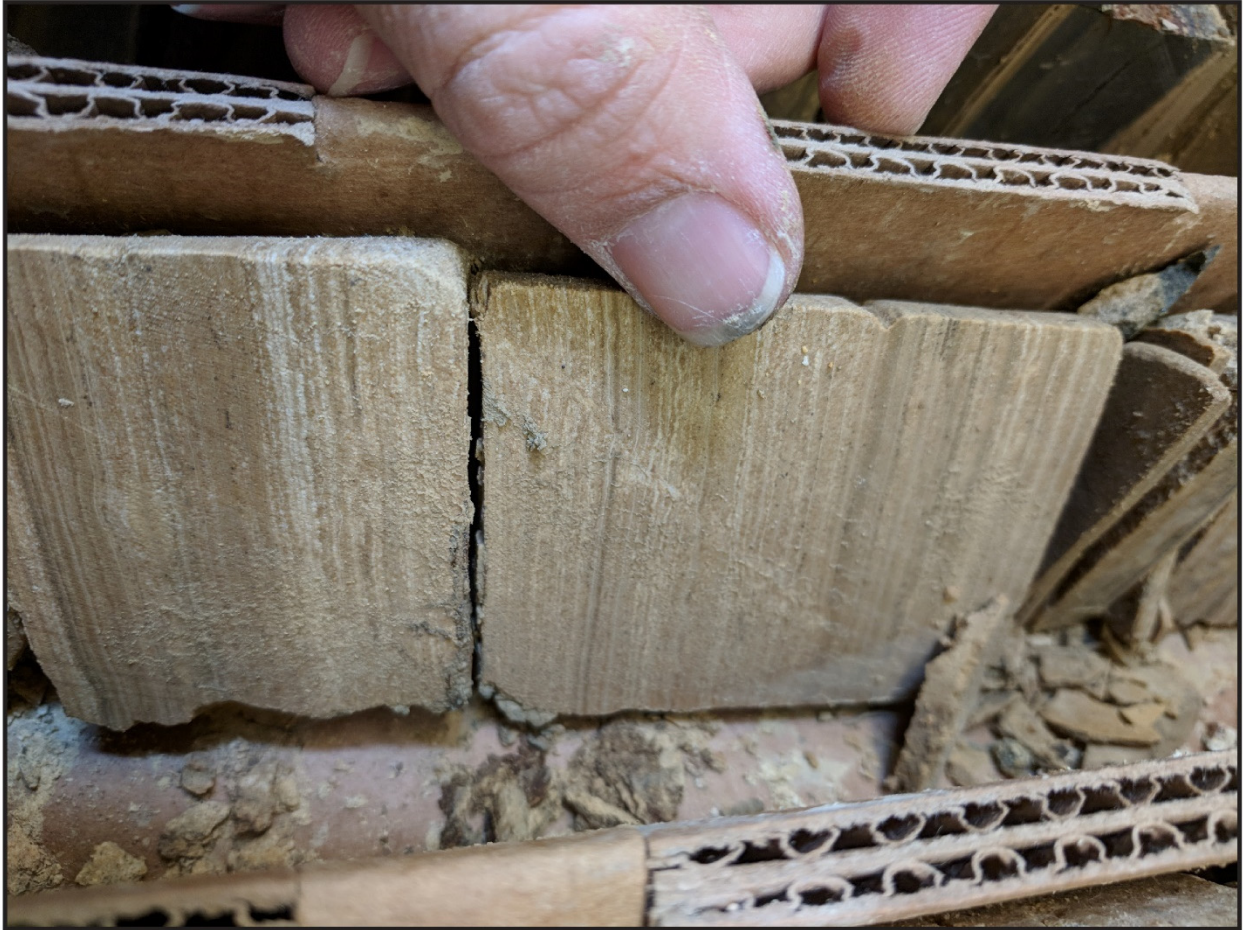
Figure 11-2 Half Core Sawed by a Diamond Blade
